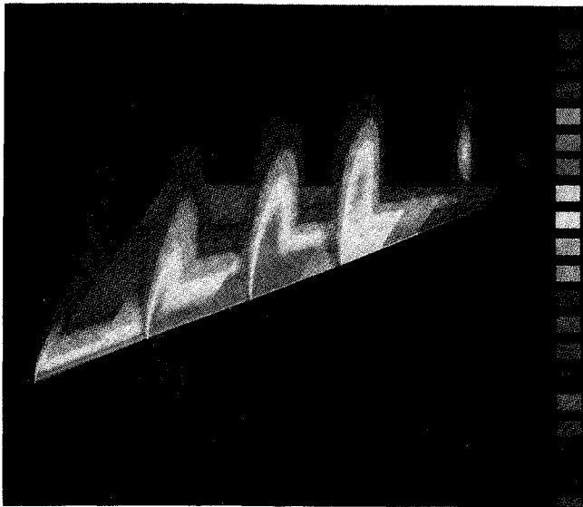
Fig. 14 Flowfield and wing surface color shaded according to pressure for a cropped delta wing, M = 0.6 and \alpha = 15 deg, (blue: low, red: high).
